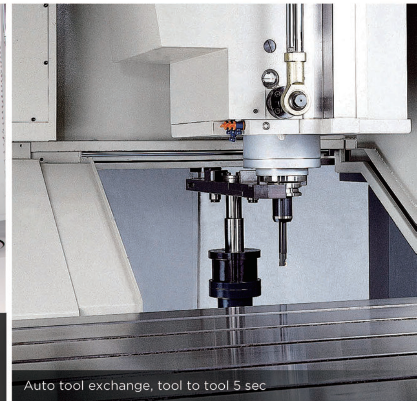
Side-mount tool magazine to save floor space, 32 tools magazine, 40 or 60 tools magazine(opt.) Random tool change and special tool management
